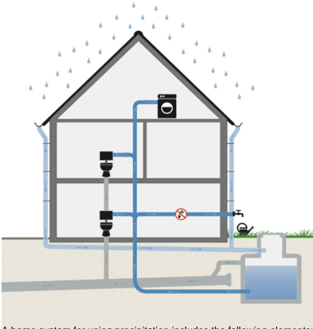
A home system for using precipitation includes the following elements: a reservoir, a pump, a connection to points of use, an overflow and a top-up system. The benefit of such a system is that the dimensions of the reservoir content can be matched to the amount of precipitation available and/or the projected use.
